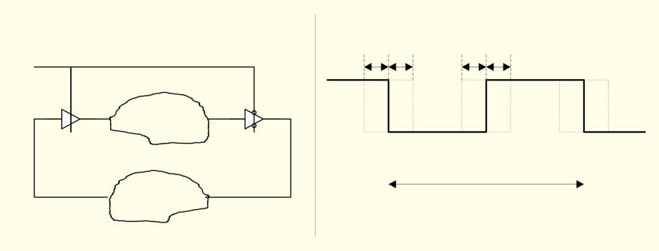
Nominal time, t=0 is set at the leading edge of the clock. The latest allowed data arrival times into latches L1 and L2, respectively:
