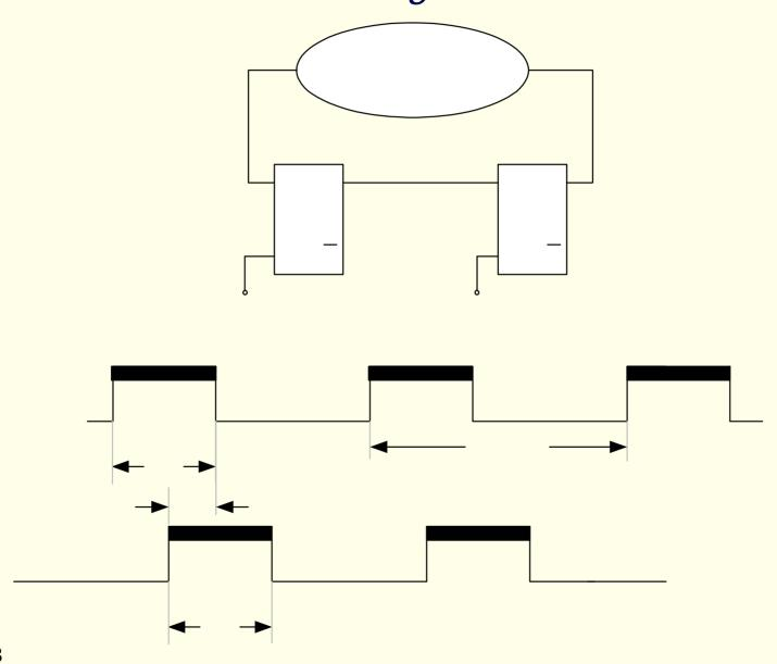
From the latest signal arrival analysis, several conditions can be derived. First, we need to assure an orderly transfer into  $L_2$  Latch (*Slave*) from the  $L_1$  Latch (*Master*), even if the signal arrived late (in the last possible moment) into the (*Master*)  $L_1$  Latch. This analysis yields the following conditions:
