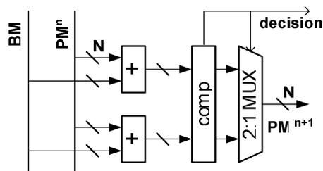
Figure 1. ACS block diagram
