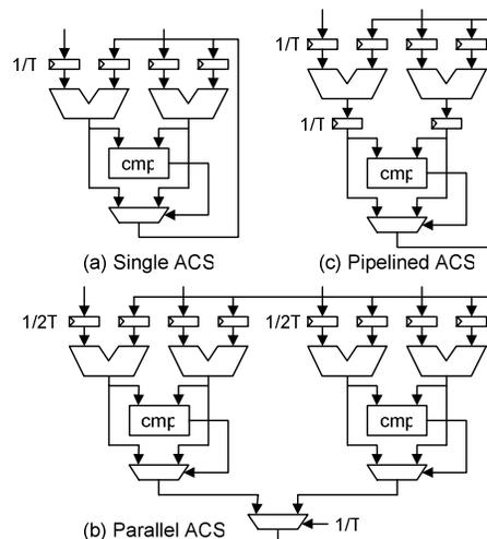
Figure 2. Architectural approaches for an ACS circuit
