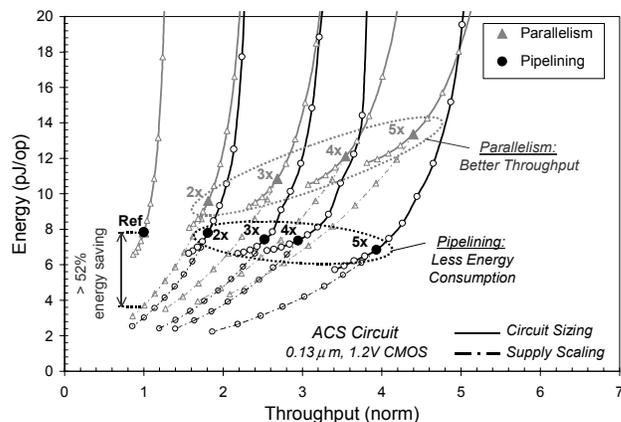
Figure 3. Energy-throughput relationship of architectures
