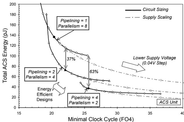
Figure 6. Energy-performance comparison of ACS units
