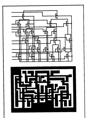
Fig. 5 Schematic and layout for bit 0 of the mod 7 multiplier
