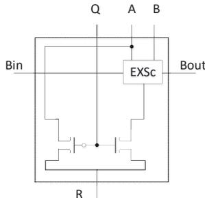
Fig. 1 An exact restoring divider cell [16].
