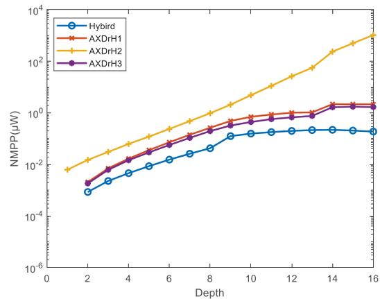
Fig. 17 NMPP of the proposed AXHD and AXDr using HR schemes at various replacement depths.
