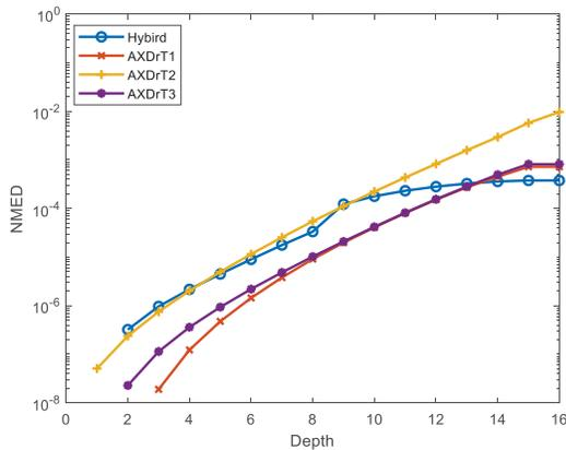
Fig. 8 The NMED of the proposed AXHD and AXDrs using TR schemes for various replacement depth.
