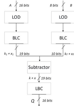
Fig. 3 A 16 by 8 unsigned non-iterative logarithmic divider [10].
