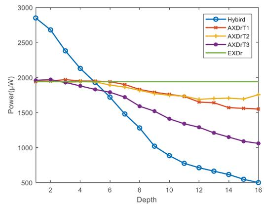
Fig. 10 Power of the proposed AXHD, EXDr, and AXDrs using TR schemes at various replacement depths.
