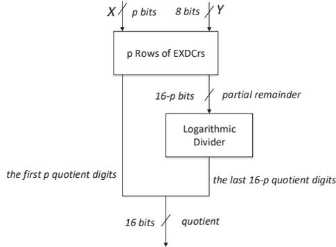
Fig. 4 16 by 8 AXHD based on restoring and logarithmic dividers.
