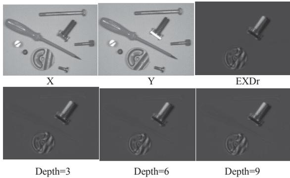
Fig. 19 Change detection using EXDr and AXHDs.
