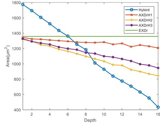
Fig. 13 Area of the proposed AXHD, EXDr, and AXDRs using HR schemes at various replacement depths.
