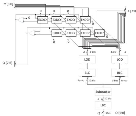
Fig. 5 8 by 4 AXHD based on restoring and logarithmic dividers for  $p=2$ .
