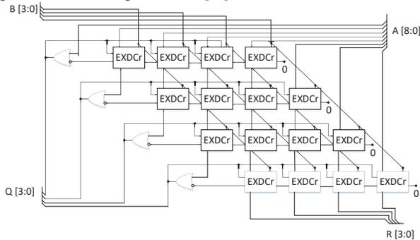
Fig. 2 A conventional unsigned 8 by 4 restoring array divider [16].
