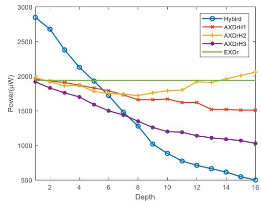
Fig. 9 Power of the proposed AXHD, EXDr, and AXDrs using HR schemes at various replacement depths.
