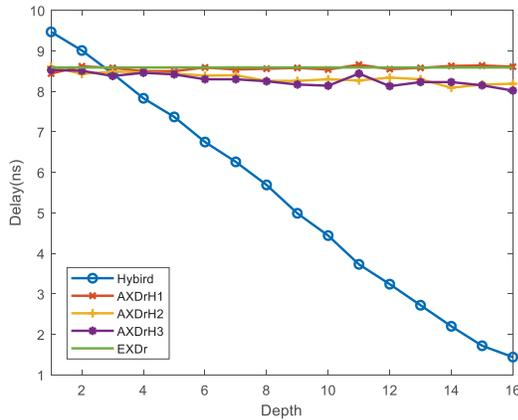
Fig. 11 Delay of the proposed AXHD, EXDr, and AXDRs using HR schemes at various replacement depths.
