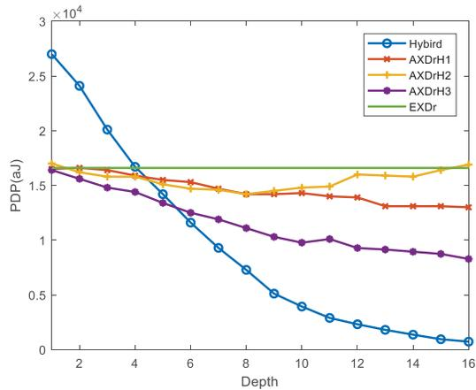
Fig. 15 PDP of the proposed AXHD, EXDr, and AXDr using HR schemes at various replacement depths.
