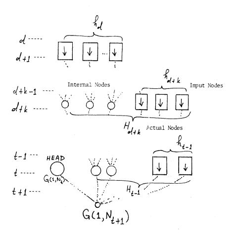
Fig. 2: The general computation tree of  $G(1,N_{t+1})$  Arrow at d+k level indicates a (d+k)-maximal which is ANDed by an appropriate propagating function.
