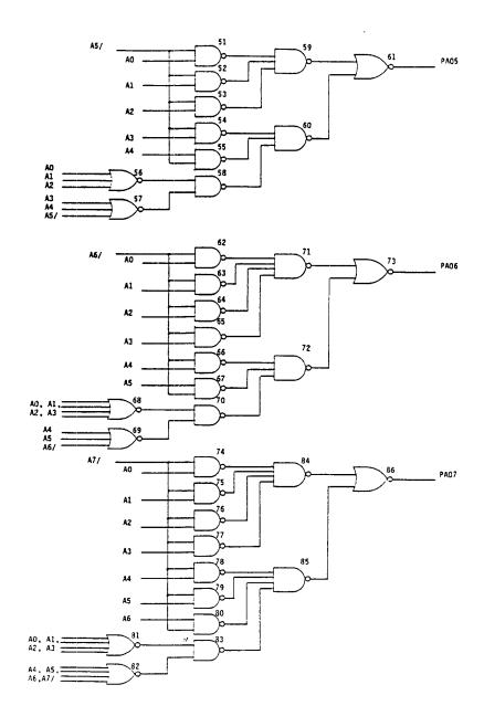
Figure 6 Circuit diagram of the MDL module (a submodule of Modulo P Adder)
